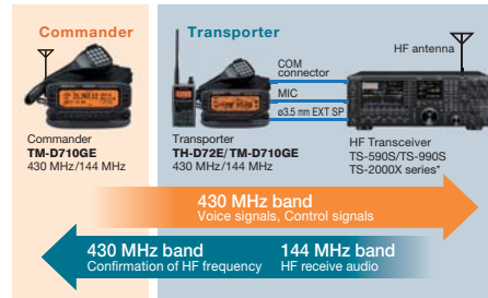
KENWOOD SKY COMMAND SYSTEM II uses a pair of TH-D72E/TM-D710GE transceivers.
